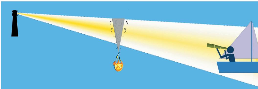
A third effective technique used to ignore light from external influences is to focus the receiver to observe only the transmitter – rather like a sailor who uses a telescope to observe the flashing of a distant lighthouse. The disadvantage of this approach is that the telescope must be carefully and consistently aligned. Hence OSID does not use this technique.
