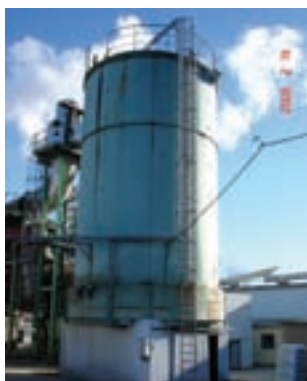
Figure 4, left: the 300 m 3 test silo used for the gas distribution tests. Right: simulated nitrogen distribution inside the test silo assuming a higher amount of fine fraction in the silo centre and an injection rate of 4.5kg/m 2 h. Red colour – 100 % N 2 , blue colour – air (21% O 2 ). The silo centre and the gas inlet are located in the lower left corner of the figure.
