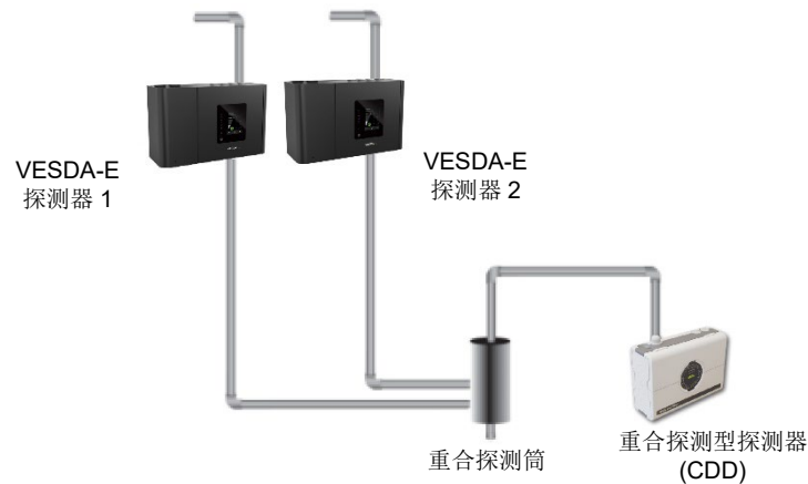
图 27: VESDA 排气采样重合探测选项的探测器布置
