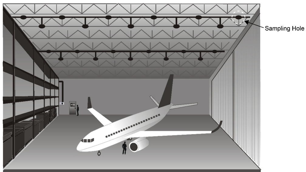
Figure 1: VESDA high-low alternating ceiling detection in Aircraft Hangar
