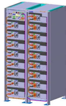
Air-cooled CATL (Equivalent to 2x battery rack)
