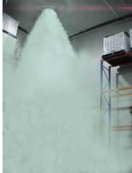
After the sprinkler was turned off, all the water had accumulated on the floor and turned to black ice. Concerns were raised in regards the safety of fire brigade personnel. This further highlights that a reliable and very early warning smoke detection technology is highly desirable in refrigerated storage facilities.
