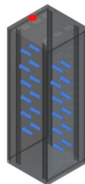
Figure 2: Monitoring Sensor Placement Above Racks - Mounted to Walls
