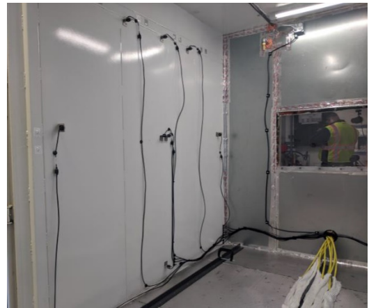
Figure 8: Large-Scale Fire Testing Enclosure Outfitted with Several Sensors
