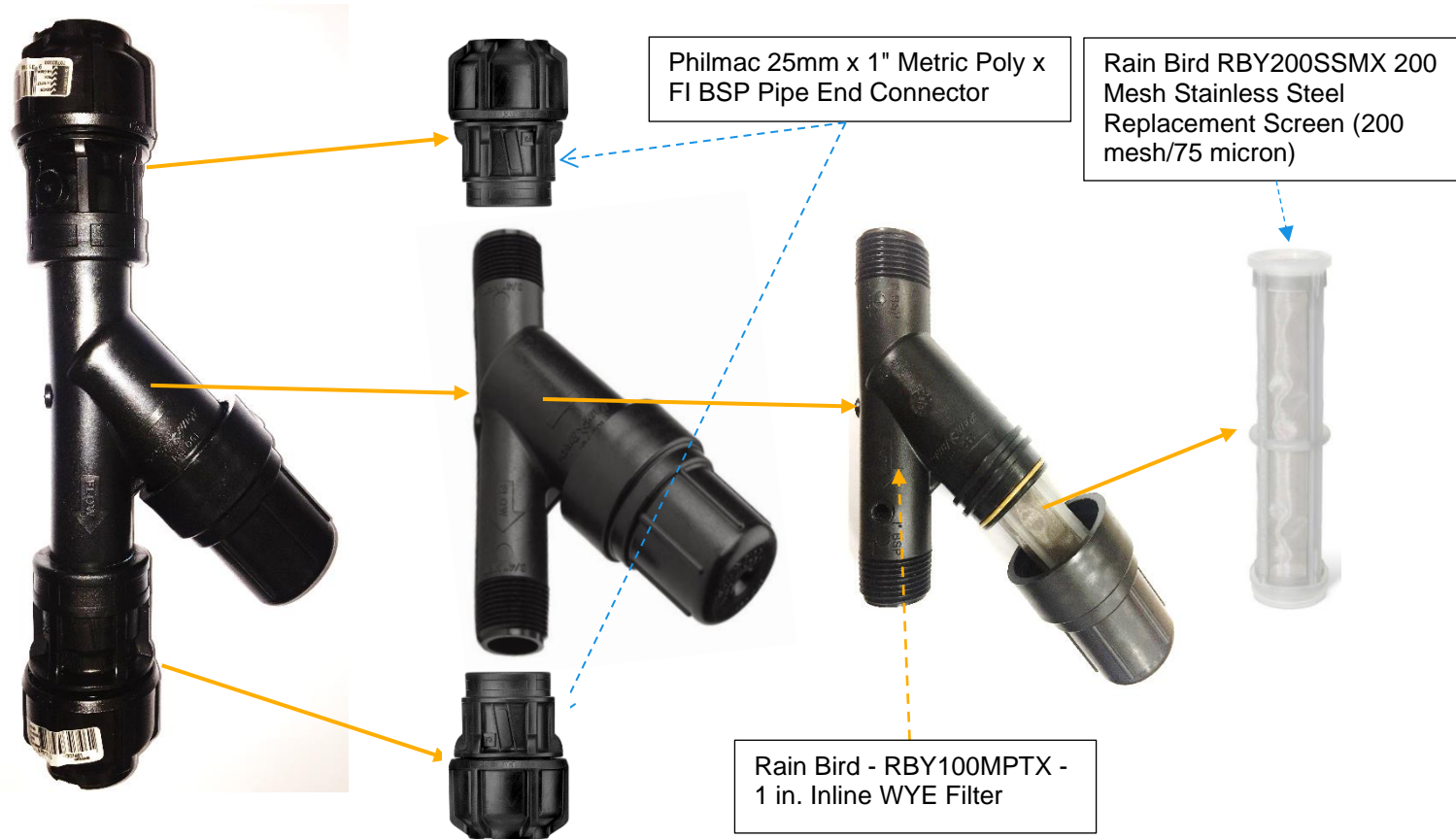
Figure 1: In-Line Mesh Strainer Assembly
