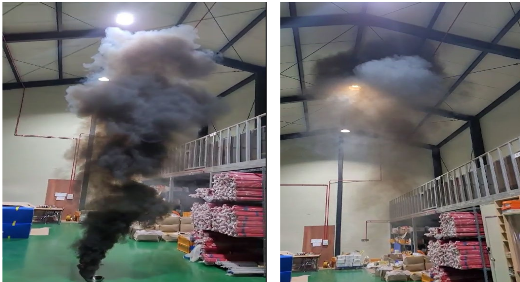
Figure 3: Smoke Testing Within WINETCH Warehouse
