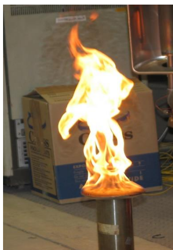
Figure 5: N-Heptane Fire Test
