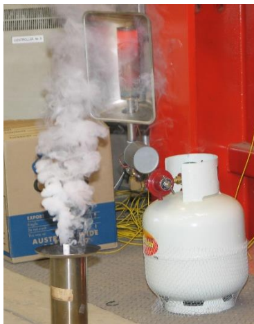
Figure 4: Smoke Pellet Test
