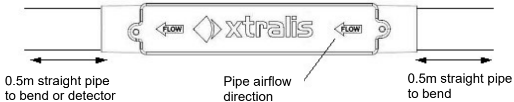
Figure 2: Xtralis In-Line Filter (Top View) – Horizontal Installation
