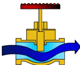
Gate Valve Opened
