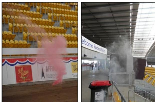
Following the smoke testing a pipe network design was prepared. A total of seven VESDA VLI detectors were required. A greater concentration of sampling points was included, considerably more than the number of point detectors installed in the original fire detection system to cover the same area.
