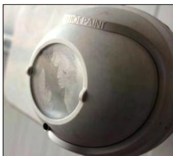
Water condensing on an Imager or Emitter is the result of their surfaces' temperature cooling below the dewpoint of the air which is in contact with them.
