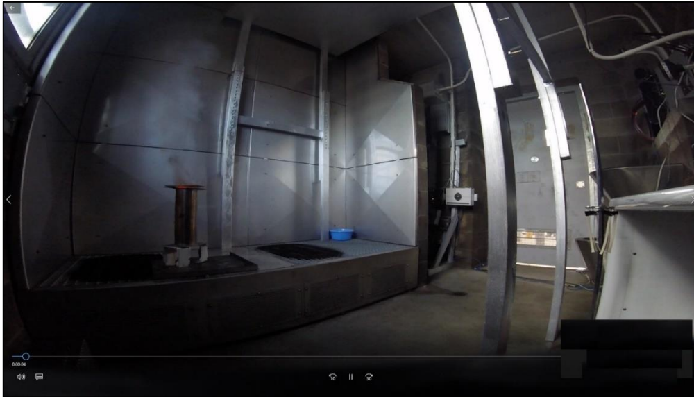
Figure 5: newsprint burning – captured by the video camera
