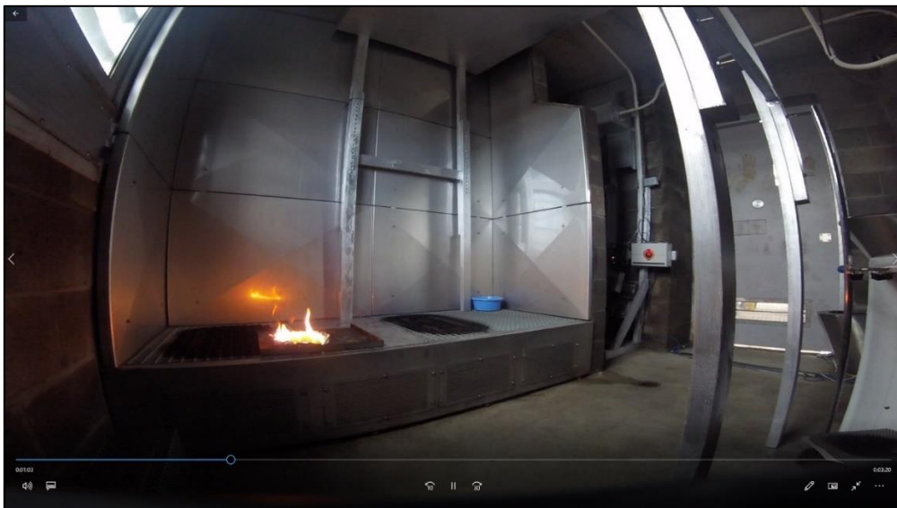
Figure 4: PU foam fire – captured by the video camera
