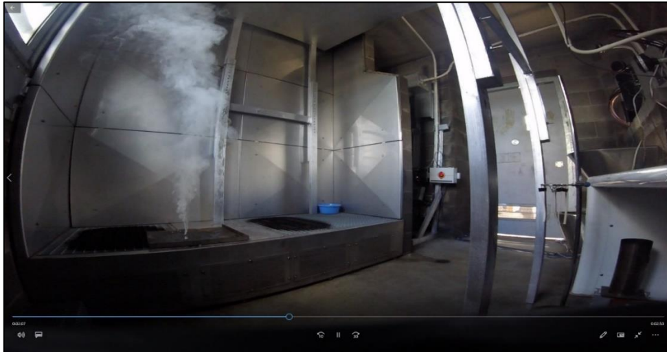
Figure 7: Smoke pellet burning – captured by the video camera
